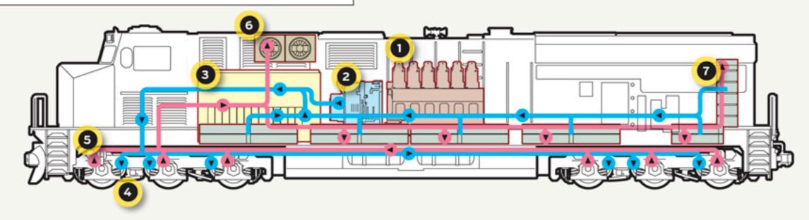
GE's hybrid concept is modeled on the Evolution locomotive, but—like a hybrid car—it stores energy generated when the brakes are applied.
