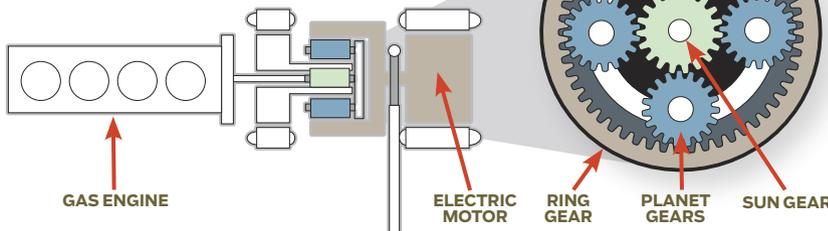
Toyota Prius's planetary-gear torque splitter proportions power between the electric motor, engine and front wheels. This allows the engine or motor, or both, to drive wheels, while the engine or wheels can power a generator to charge batteries. This device also acts as a constantly variable transmission.
