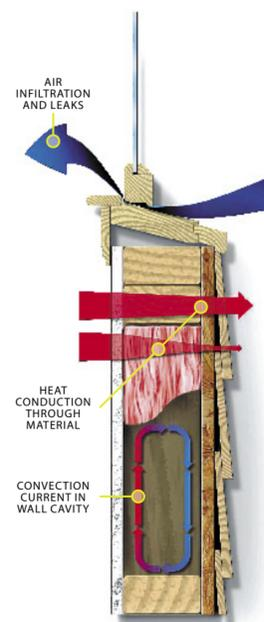
**DRAFTS:** In winter, cold air infiltrates around doors and windows, and through gaps in the walls. Warm air can escape through flues and around vents.
