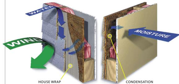
on batts or plastic films, to control the problem. Special care must be taken around windows and other breaks to avoid excessive moisture that causes rot. To control drafts, house wrap goes on the outside. This material is waterproof, yet vapor-permeable so it won't lock moisture in the wall cavities.
